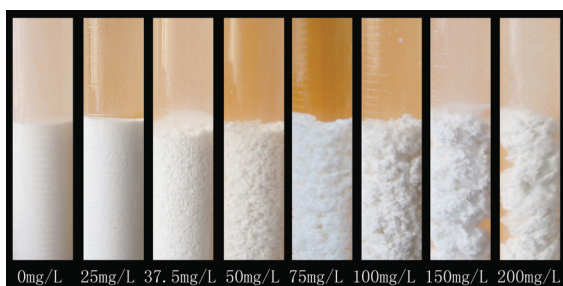
图3 不同浓度非离子聚丙烯酰胺作用 \text{TiO}_2 纳米酶的絮凝沉降图 Figure 3 Digital photograph of flocculation and sedimentation behaviour of \text{TiO}_2 -enzyme microflocules at different concentrations of nPAM
