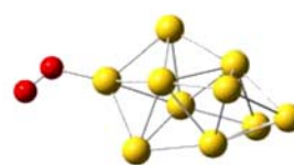
图 3 MP2 计算 \text{Au}_{10}\text{-O}_2 配合物的结构 Figure 3 Complex geometry of \text{Au}_{10}\text{-O}_2 , calculated at the MP2/6-311G(d) level
