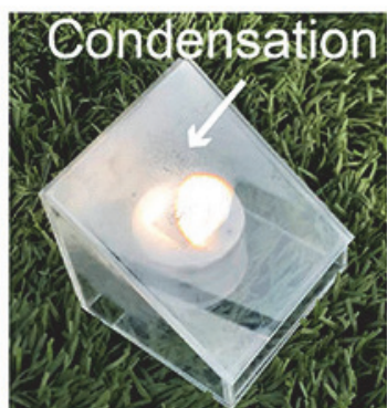
图2 实际阳光照射下太阳能驱动海水淡化试验的光学照片 Figure 2 The optical photographs of the solar-driven desalination test under the actual sunlight irradiation Reprinted (Adapted or Reprinted in part) with permission from {ACS Nano 2022, 16, 2511.}. © {2022} American Chemical Society
