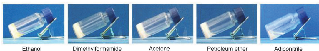
Figure 4 Responsive properties of organic solvents for the hydrogel SH-BP5 ( w = 2.0\% , \lambda_{\text{ex}} = 340 \text{ nm} , M / BP5 , 1 : 0.5 in molar ratio)
